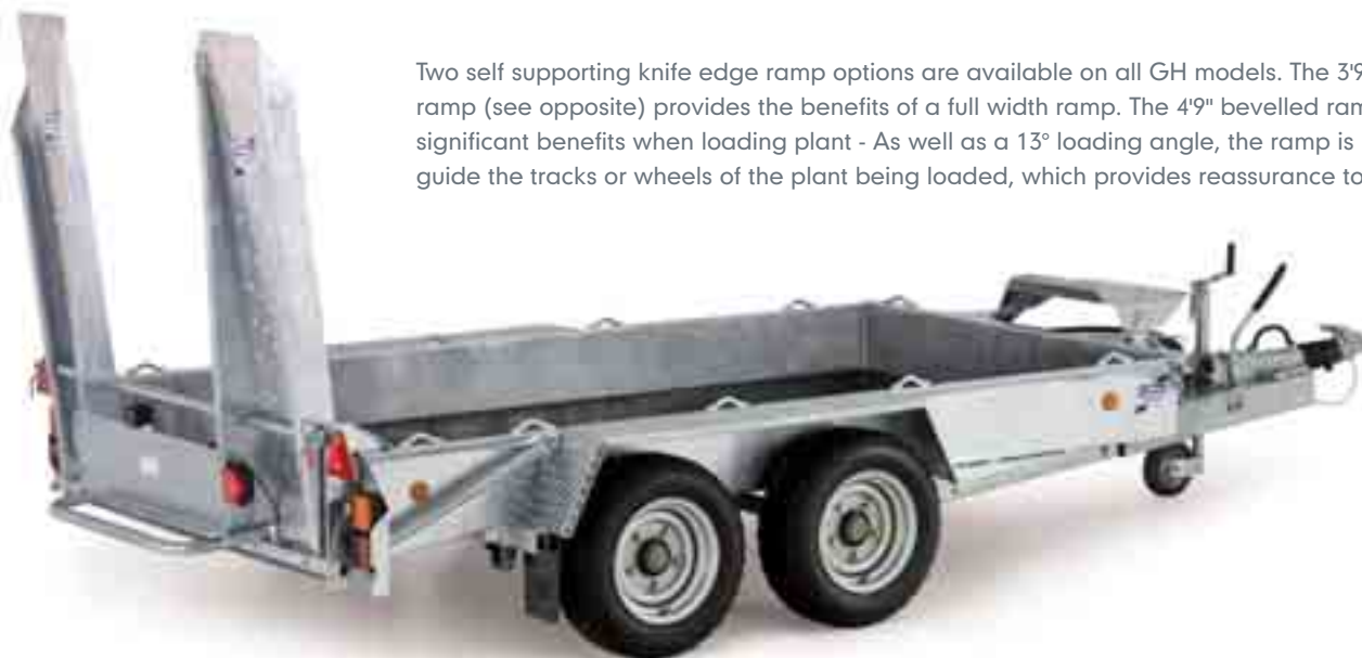
GH1054 with 4'9" bevelled ramp
